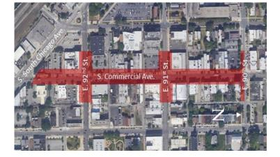
Commercial Ave will be improved as the City renovates this street with infrastructure improvements. The project will consist of numerous improvements, including fullwidth roadway resurfacing, new curb and gutter, drainage improvements, new sidewalks, parkway pavers, new roadway lighting, and new street trees.
