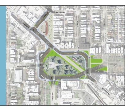
The fourth concept is called Two-Way, The Bend. Two-Way, The Bend realigns Kedzie Avenue west of the CTA station to create a new public space to the east. The concept "bends" Milwaukee Avenue around the north and east sides of the square to create one larger public space. The streets on the west and south sides of the Square to are converted to two-way traffic.
