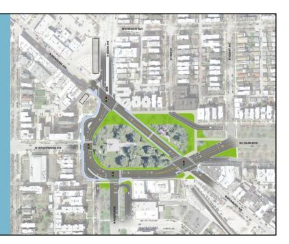
The third design concept is called Two-Way, Trip Match. Two-Way, Trip Match maintains Kedzie Avenue east of the CTA terminal and Milwaukee Avenue through the Square. The main change from existing conditions is that the streets on the west and south sides of the Square are converted to two-way traffic and the roadway on the north side of the square is converted to park area.
