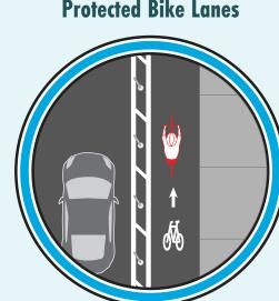
Protected bike lanes physically separate people on bikes from motor vehicle traffic through the use of vertical elements such as on-street parking, bollards, and/or raised curbs.
