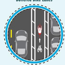
A portion of the roadway designated by striping, signing, and pavement markings for the preferential or exclusive use of people riding bikes. Buffered bike lanes provide additional marked buffer space on one or both sides of the bike lane to provide greater separation from adjacent travel and parking lanes.
